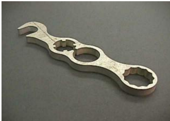
Different engineering components machined with AWJ
